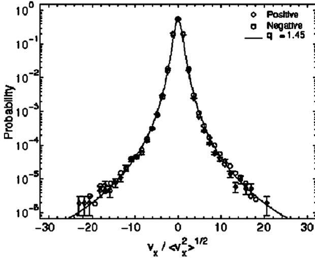
Figure 6. Measured probability density of defect velocities and fit with a  $q$ -Gaussian with  $q = 1.45$ .
