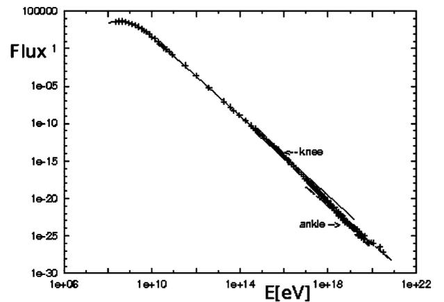
Figure 4. Measured energy spectrum of cosmic rays and a fit by Equation (85) with  $q = 1.215$ . The ‘knee’ and ‘ankle’ are structures that go beyond the simple model considered here.
