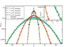
green lines represent the CTRW theory pdf for  $\gamma = 0.95$ : corrects the mismatch to Gaussian in the tails
