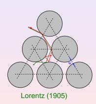
moving point particle of unit mass with unit velocity scatters elastically with hard disks of unit radius on a triangular lattice only nontrivial control parameter: gap size w paradigmatic example of a chaotic
