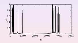
phenomenology of intermittency: long periodic laminar phases interrupted by chaotic bursts; here due to an indifferent fixed point, M'(0) = 1 (Pomeau, Manneville, 1980)
